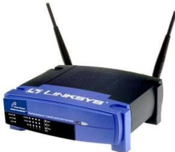
Fig 2.7 Wireless Access Point
